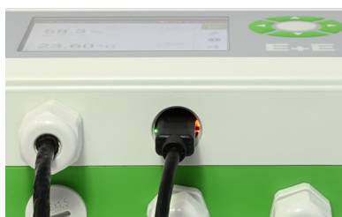
Fig. 41 Plugged USB cable and LED indication
