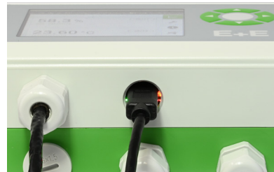
Fig. 20 Plugged USB cable and LED indication
