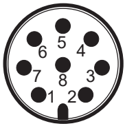
EE364 M12 device plug front view
