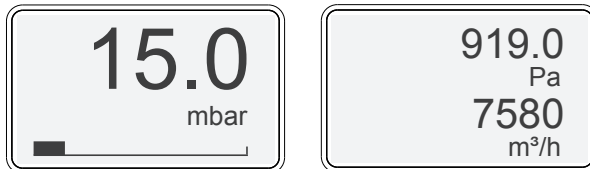
Fig. 12 Display with one line with limit bar and two lines without limit bar
