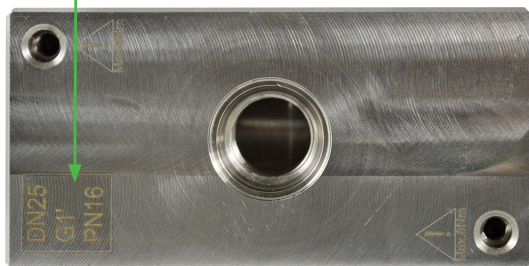
Fig. 3 Pipe diameter on gauge mounting block
