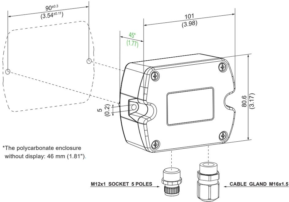
Fig. 1 Sigma 05 dimensions in mm (inch)
