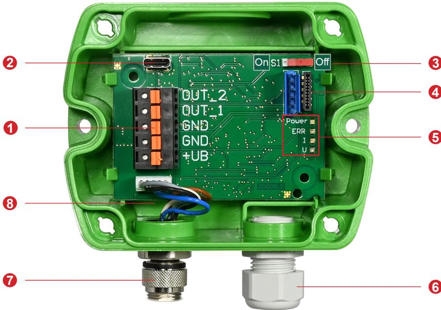
Fig. 3 Sigma 05 electronics board
