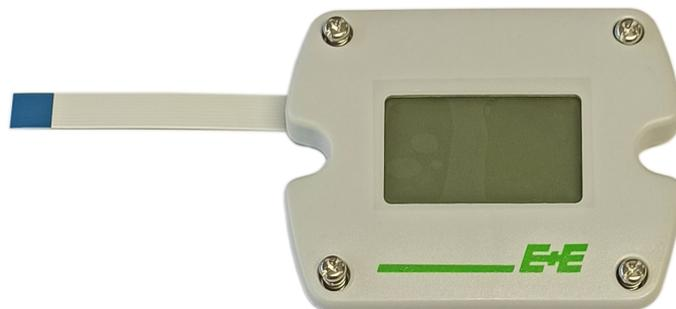
Fig. 8 FFC cable connection on the Sigma 05 electronics board
